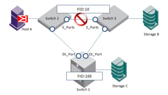
Referring to the exhibit, FC-FC routing has been properly configured. The ISL has failed.
