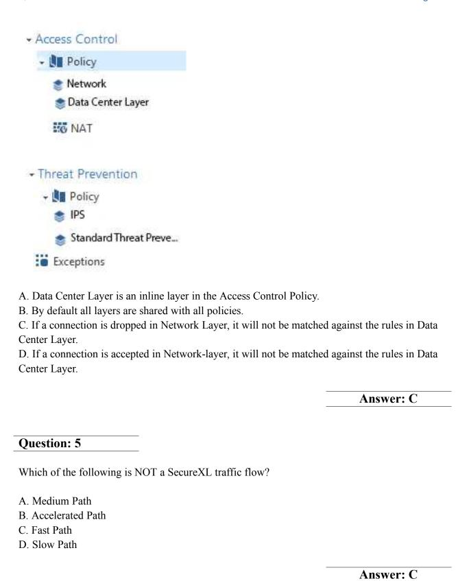
SecureXL is an acceleration solution that maximizes performance of the Firewall and does not compromise security. When SecureXL is enabled on a Security Gateway, some CPU intensive operations are processed by virtualized software instead of the Firewall kernel. The Firewall can inspect and process connections more efficiently and accelerate throughput and connection rates. These are the SecureXL traffic flows:
