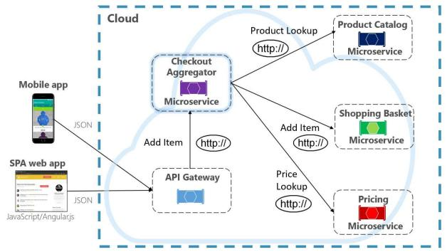
The pattern isolates an operation that makes calls to multiple back-end microservices, centralizing its logic into a specialized microservice. The purple checkout aggregator microservice in the previous figure orchestrates the workflow for the Checkout operation. It includes calls to several back-end microservices in a sequenced order. Data from the workflow is aggregated and returned to the caller. While it still
