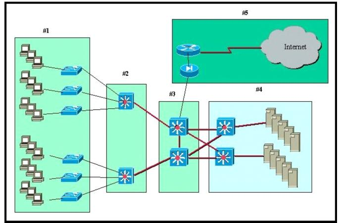
A standard Layer 2 campus network design is pictured. Which numbered box represents the core layer?
