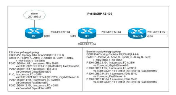
Users in the branch network of 2001:db8:0:4::/64 report that they cannot access the Internet. Which command is issued in IPv6 router EIGRP 100 configuration mode to solve this issue?
