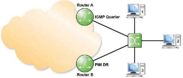
The switch is not igmp-snooping/proxy capable. What will happen if host 2 issues an IGMP report to join a group?
