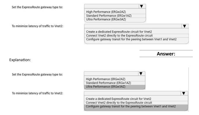
For the first question, only ExpressRoute GW SKU Ultra Performance support FastPath feature. For the second question, vnet1 will connect to ExpressRoute gw, once Vnet1 peers with Vnet2, the traffic from on-premise network will bypass GW and Vnet1, directly goes to Vnet2, while this feature is under
