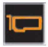
A customer notices that an indicator on the left control panel of the PowerEdge Server has turned solid amber.
