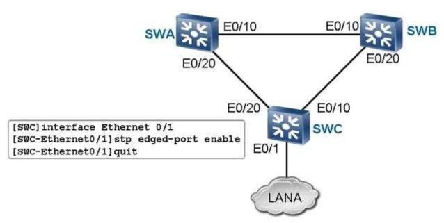
On the RSTP network as shown in the figure, what is the port role of SWC E0/1 according to the configuration? (Select 2 Answers)
