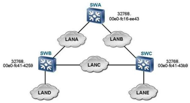
As shown in the figure, when the STP network runs properly, which device does the designated port of LANC reside?
