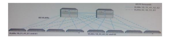
The exhibit shows a network with HP 3500 yl Series switches at the access layer and HP 8206 zl switches at the core. The customer with this solution has logged several support calls, which were eventually tracked down to spanning tree issues. How can a network architect adjust the solution to prevent the issue in the failure?
