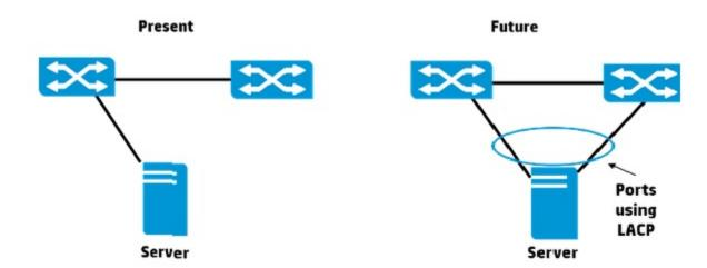
The exhibit shows the physical connection between two HP Comware switches and a server The network administrator is concerned about redundancy and wants to implement a solution like that shown on the right side of the exhibit. The administrator plans to use an LACP link aggregation with both links active. What must the administrator do first?
