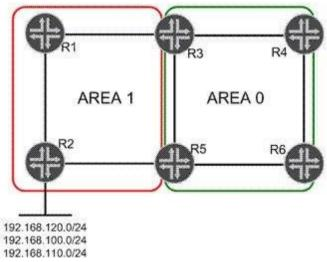
In the exhibit, Area 1 is a not-so-stubby area. Three networks are redistributed into Area 1 on R2. You must summarize the redistributed network addresses in Area 1 so that only one network prefix is readvertised into Area 0. You must also summarize the loopback addresses of R1 and R2 into a single address in Area 0.Which configuration sample on R3 and R5 will complete this task?
