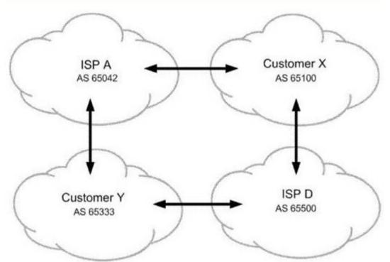
All networks shown in the exhibit contain more than one BGP speaking router. You operate ISP A. You must ensure that customer Y sends their traffic to you over the directly connected link but customer Y is not used for transit into your network. What do you do to accomplish this?
