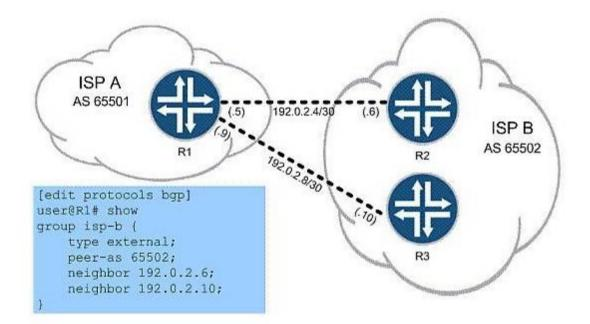
In the exhibit, ISP A is charged a higher rate for traffic sent to R2. You are asked to lower costs for ISP A by configuring R1 to send traffic to R3 whenever possible. What are two ways to do this? (Choose two.)
