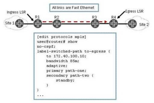
As shown in the exhibit, you have an adaptive LSP that requires 85 Mbps. The LSP is configured with a primary path and a secondary path in standby mode. All connections in the MPLS network are Fast Ethernet. Which statement is correct?
