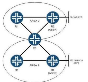
You are asked to configure an OSPF network based on the topology shown in the exhibit. You must keep the link-state database in Area 1 as small as possible. What will accomplish this?
