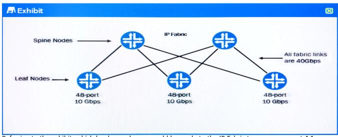
Referring to the exhibit, which hardware change would be made to the IP Fabric to ensure an exact 4:1
