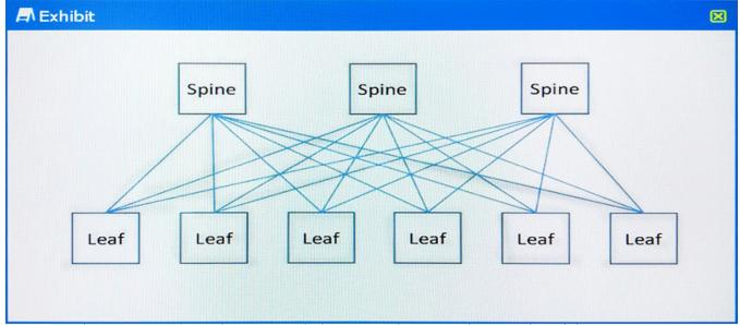
A customer has a 3-stage Clos architecture with three spine devices as shown in the exhibit.
