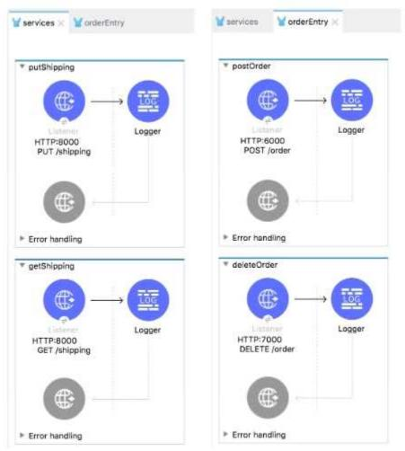
The two Mule configuration files belong to the same Mule project. Each HTTP Listener is configured with the same host string and the port number, path, and operation values are shown in the display names.
