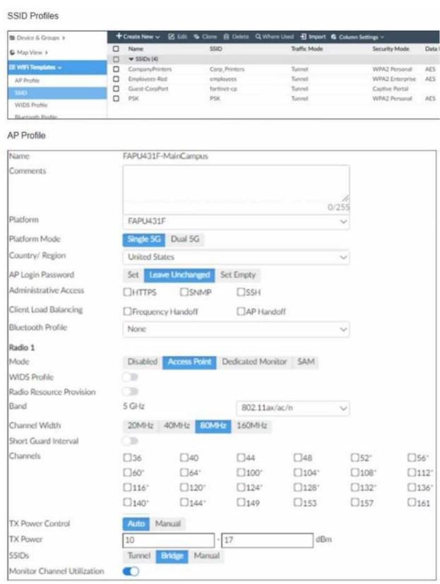
The exhibits show the wireless network (VAP) SSID profiles defined on FortiManager and an AP profile assigned to a group of APs that are supported by FortiGate
