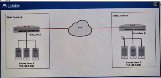
Your company has two data center (DC) connected using a Layer 3 network. Service in farm A need to connect to server in farm B as though they all were in the same Layer 2 segment.
