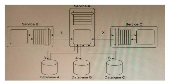
Service A is an entity service that provides a set of generic and reusable service capabilities. In order to carry out the functionality of any one of its service capabilities, Service A is required to compose Service B (1) and Service C (2), and Service A is required to access Database A (3), Database B (4), and Database C (5). These three databases are shared by other applications within the IT enterprise.
