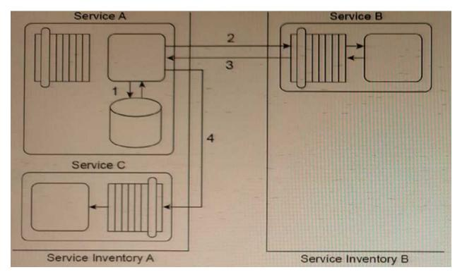
Service A is a task service that sends Service B a message (2) requesting that Service B return data back to Service A in a response message (3). Depending on the response received, Service A may be required to send a message to Service C (4) for which it requires no response.
