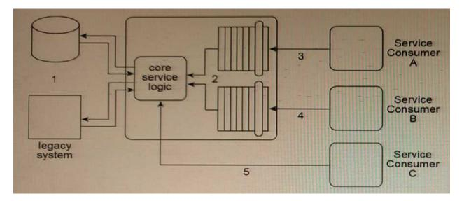
The architecture for Service A displayed in the figure shows how the core logic of Service A has expanded over time to connect to a database and a proprietary legacy system (1), and to support two separate service contracts (2) that are accessed by different service consumers.
